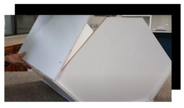
4. Place in one of the remaining rear side panel pieces and screw it in place, using the pre-drilled holes as a guide. Repeat the same for the other rear side panel.
