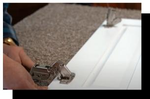
15. Flip down and expand out the hinges attached to the door before aligning the hinge to the holes on the cabinet frame's wood blocks and screwing it on. If you wish for the door to open to the left, attach the hinge to the left side blocks. For it to open to the right, attach to the right side blocks.
