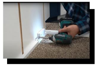
5. Further secure the side panel to the frame using the provided metal L brackets, placing one at the top and one at the bottom of the frame. Repeat steps 3 - 5 for the other frame and front side panel piece. Making sure to that the grooves of the two pieces line up to each other before securing in place.
