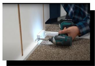
3. Further secure the side panel to the frame using the provided metal L brackets, placing one at the top and one at the bottom of the frame. Repeat steps 2 - 3 for the other frame and front side panel piece. Making sure to that the grooves of the two pieces line up to each other before securing in place.
