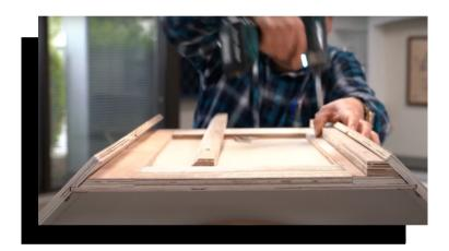
13. Next, connect the toe kick pieces together, making sure that the cut out edges are facing up before screwing in place. Secure the toe kick piece to the cabinet using a brad nails.
