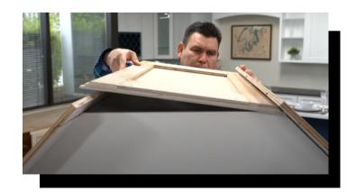
10. Use the included 135 degree metal bracket pieces to further secure the back panel piece to the rear side panels from the inside of the cabinet box.
