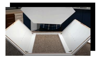
3. Next, place in the top and bottom panels following the groove lines.
