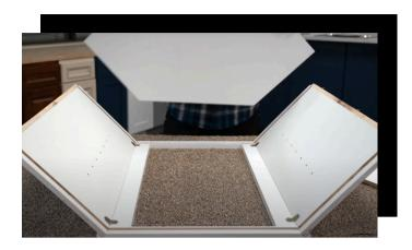
3. Next, place in the bottom panels following the groove lines.
