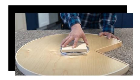
1. Take out the two revolving shelves from the separately packed "LSK" box. Taking one of the revolving shelves, flip it upside-down and turn the attached plywood piece of hardware until you hear a "click" sound indicating that the revolving shelf is set to the correct position with the protruding metal panel pointed towards the 90 degree corner.
