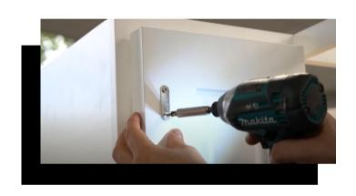
18. Repeat steps 16 - 17 for the bottom magnet pieces. Finish by adding on rubber door stoppers to the outer back corners of the door.
